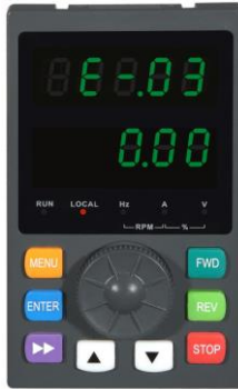
Fig. 4-5 Fault alarm display state
