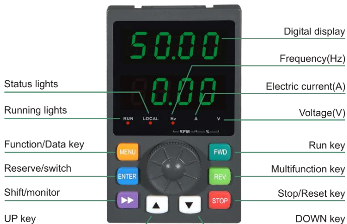
Fig. 4-3 Control panel diagram
